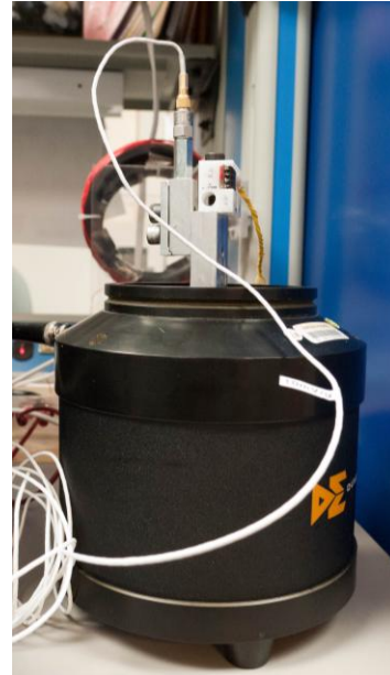
Figure 3, Sensor stick and the reference sensor on the shaker
